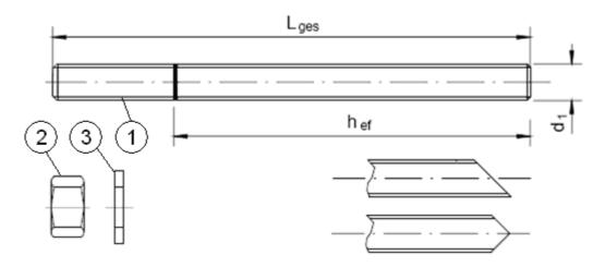
Standard commercial threaded rod with marked embedment depth
